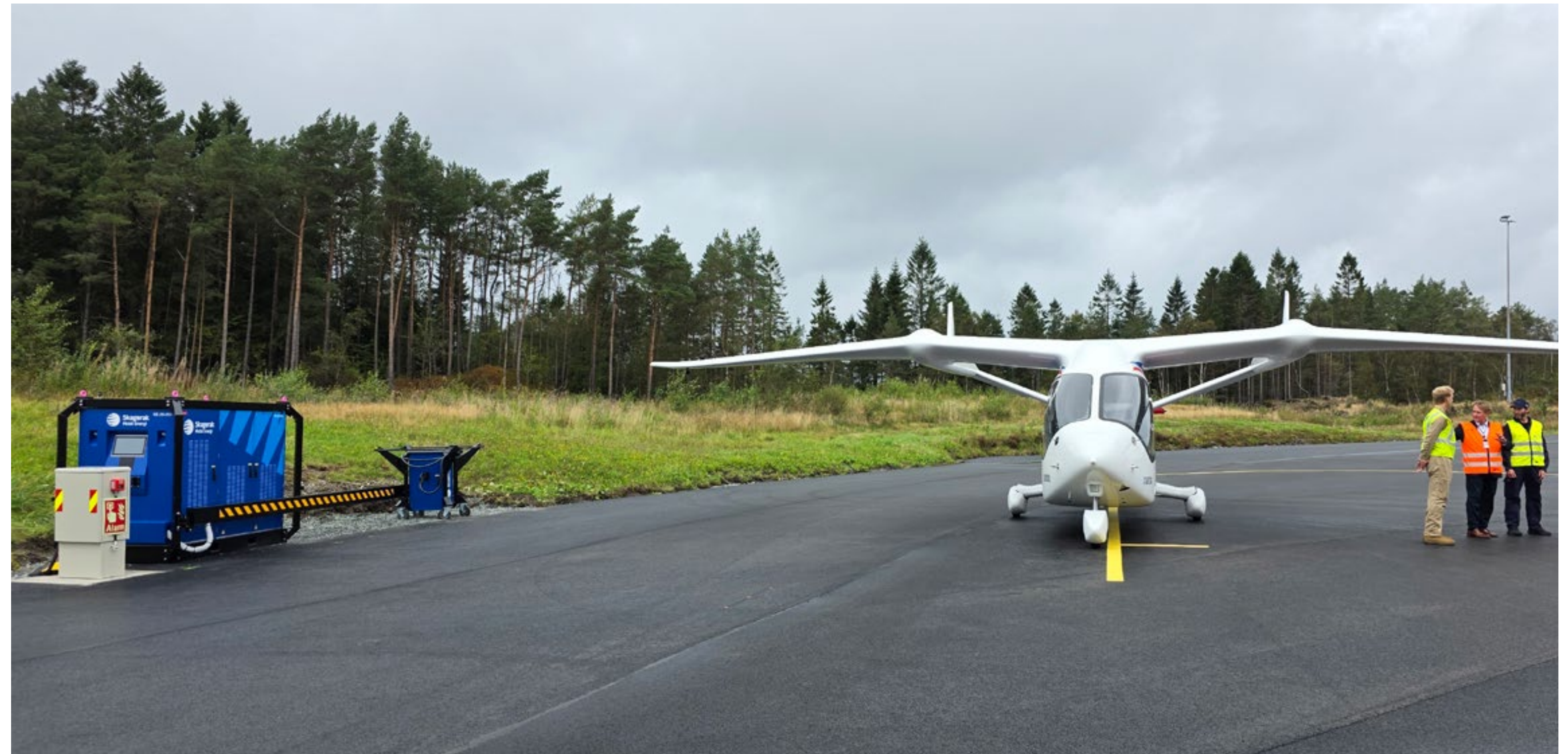
Image 8: Demonstration aircraft and temporary mobile charging infrastructure at Bergen airport. Photo: M.S. Mølmen / Avinor
